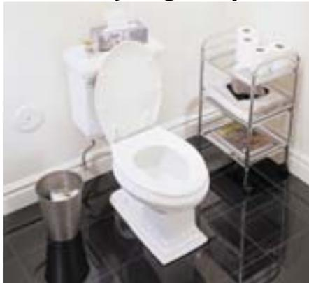
**3. Test toilets for leaks.** Add a few drops of food coloring to the water in the toilet tank, but do not flush the toilet. Watch to see if the coloring appears in the bowl within a few minutes. If it does, the toilet has a silent leak that needs to be repaired.
